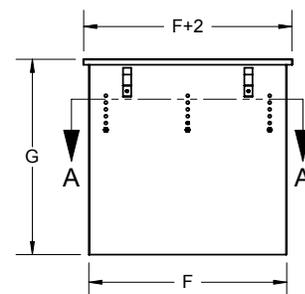
Note: Interceptor support brackets adjustable for varying depths of floor construction.
