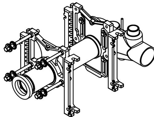
\* Recommend feet be secured to floor with 1/2 fasteners and anchors (by others).
