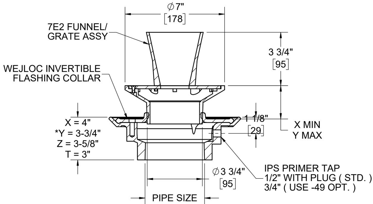
\*GASKET ON -Y CONNECTION CONFORMS WITH ASTM-C564
